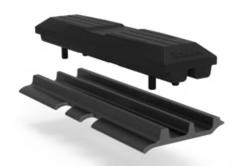
• Clip-On Track Pads. They are mounted by means of the built-in side clips, and their advantages include the quick installation and the possibility of replacing them without having to dismantle the whole steel track shoe.
